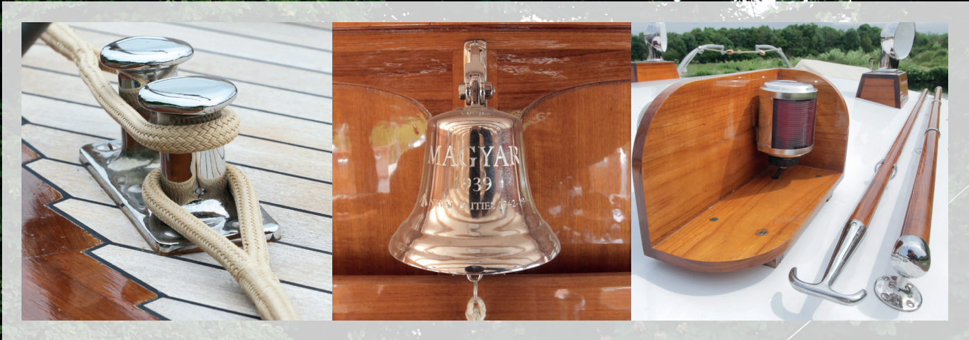
Above left to right: Bollard cleat; The original ship's bell; Port light and boat hook
